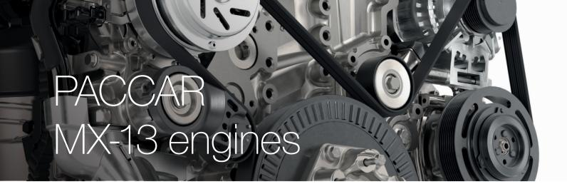
The 12.9 litre Euro 6 PACCAR MX-13 engine uses ultra-modern common rail technology, a turbo with variable geometry and advanced controls for maximum efficiency. In order to comply with the strict Euro 6 emissions requirements, it features exhaust gas recirculation, together with SCR technology and an active soot filter.
